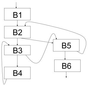
OUT[B1] = IN[B2] IN[B1] = OUT[B1] -  $\{a,b\}$ OUT[B2] = IN[B3] + IN[B5] IN[B2] =  $\{a,b\}$  + (OUT[B2] -  $\{c,d\}$ ) OUT[B3] = IN[B4] + IN[B5] IN[B3] =  $\{b,d\}$  + OUT[B3] OUT[B4] =  $\{a,b,e\}$  + (OUT[B3] IN[B4] =  $\{a,b,e\}$  + (OUT[B4] -  $\{d\}$ ) OUT[B5] = IN[B6] + IN[B2] IN[B5] =  $\{a,b,c\}$  + (OUT[B5] -  $\{e\}$ ) OUT[B6] =  $\emptyset$ IN[B6] =  $\{b,d\}$  + (OUT[B6] -  $\{a\}$ )
