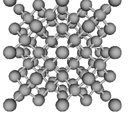
Silicon crystal seen along the <110> direction Silicon crystal seen along the <100> direction.
