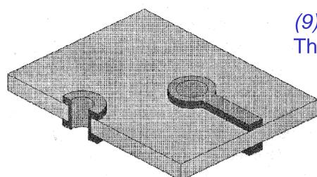
(9) Strip etch resist The tin or tin/lead is chemically removed
