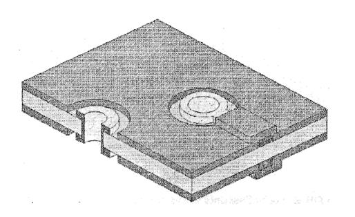
(11) Solder coat Solder (tin/lead) is applied to the exposed copper and the excess solder is removed
