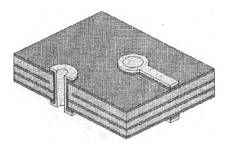
(11) Strip plating resistPlating resist is chemically removed,revealing the copper surface
