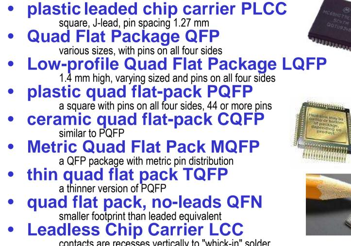
contacts are recesses vertically to "whick-in" solder. Common in aviation electronics because of mechanical endurance against vibration.
