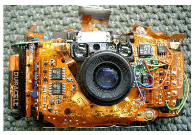
Olympus Stylus camera with skins removed, showing flex circuit assembly
