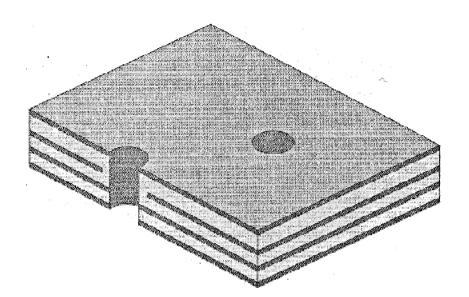
(7) Electroless copper plateA thin layer of copper is depositedfollowing smear removal, cleaning andpreparation
