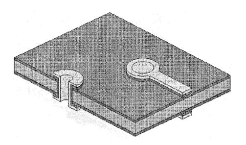
(7) Strip plating resist Plating resist is chemically removed, revealing the surface copper
