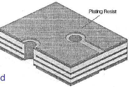
(8) Apply plating resistThe desired circuitry is left uncovered
