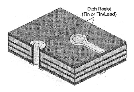
(10) Electroplate etch resistTin or tin/lead is electrolyticallydeposited over the copper plating
