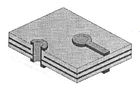
(13) Strip etch resist The tin or tin/lead is chemically removed
