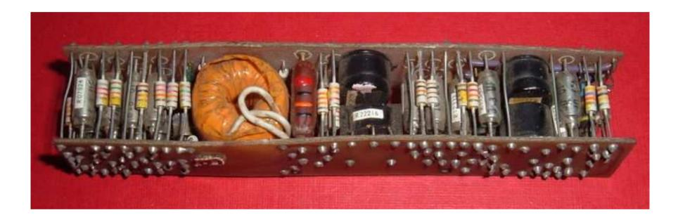
Advantages: large space-saving Application: i.e. missile guidance and telemetry systems
