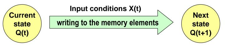
What the next state will be after the transition depends on1) the current state (values of the memory element signals Y, F)2) the values of input signals at the moment of the transition
