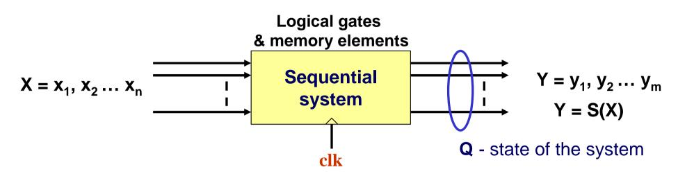
Output signals are the outputs of memory elements and they may change only after a new write operation is performed.
