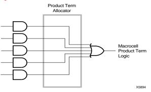
Figure 5: Macrocell Logic Using Direct Product Term
