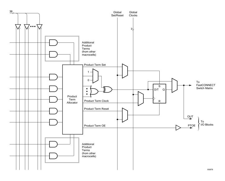
Figure 3: XC9500 Marcocell Within Function Block
