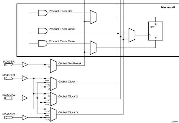
Figure 4: Macrocell Clock and Set/Reset Capability
