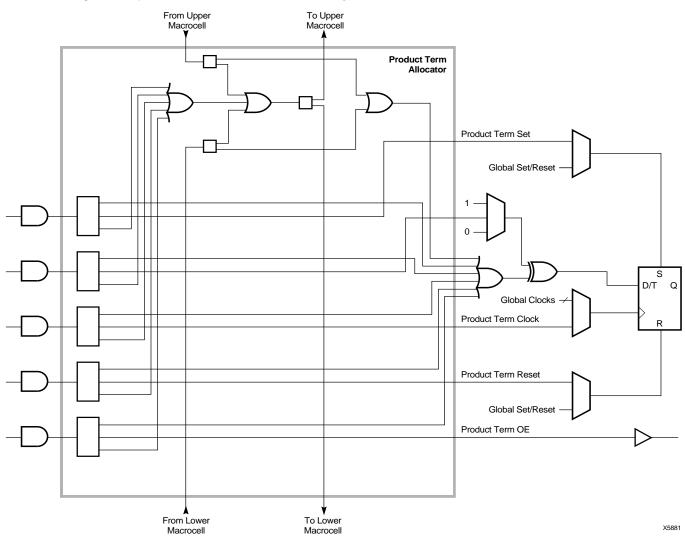
Figure 8: Product Term Allocator Logic
