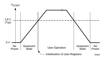
Figure 16: Device Behavior During Power-up
