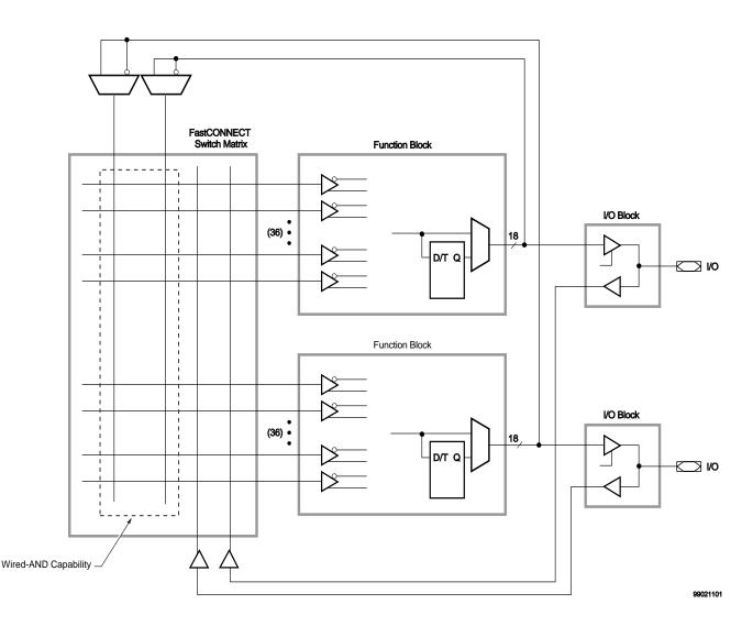
Figure 9: FastCONNECT Switch Matrix
