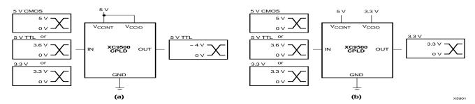
Figure 12: XC9500 Devices in (a) 5 V Systems and (b) Mixed 3.3 V/5 V Systems
