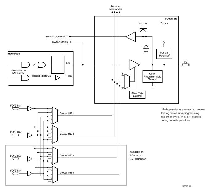
Figure 10: I/O Block and Output Enable Capability
