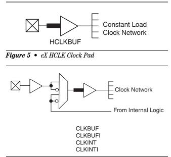
Figure 6 • eX Routed Clock Buffer
