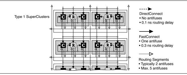
Figure 4 • DirectConnect and FastConnect for Type 1 SuperClusters
