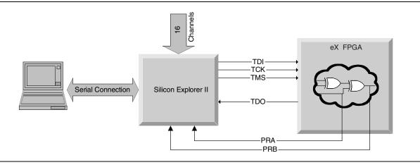
Figure 7 • Probe Setup
