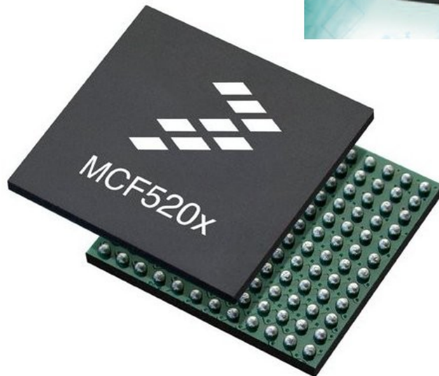
Mikrokontroler Freescale, MCF520x, BGA 256
