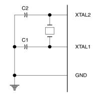
Note: C1, C2= 30 pF  $\pm$  10 pF for Crystals = 40 pF  $\pm$  10 pF for Ceramic Resonators
